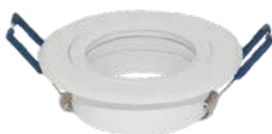
R212 WN717 White • Flat Top • Fixed CNC Aluminium Ø80 x H25 / Cut 65 - 70
